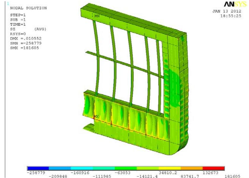
Equivalent stress distribution for internal structure
