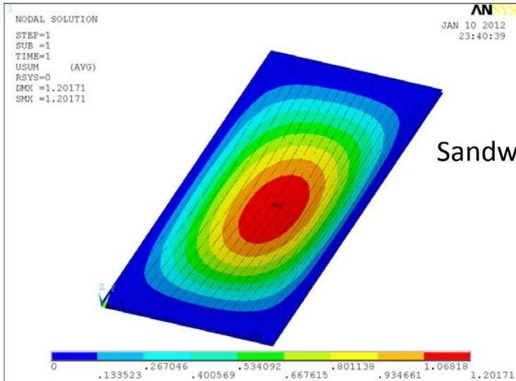
Correction factor obtained for maximal nodal displacement resemblance for this case is  $k = 8.4$
