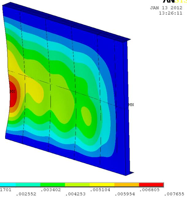
Nodal displacement output results, uncorrected
