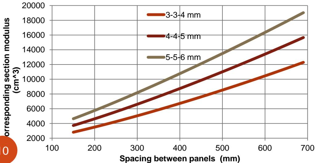
**The principle for dimensioning the double sandwich structure:**
