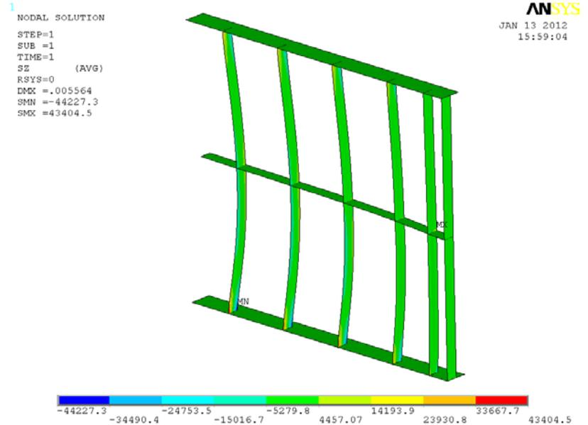
Shear stress distribution for internal structure
