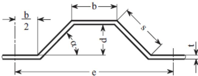
Fig. 11.2 Element of a corrugated bulkhead
