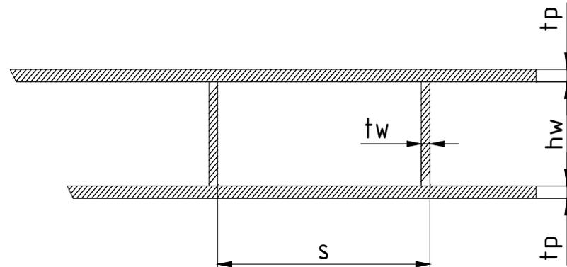
**Steel sandwich panel core configurations –**
