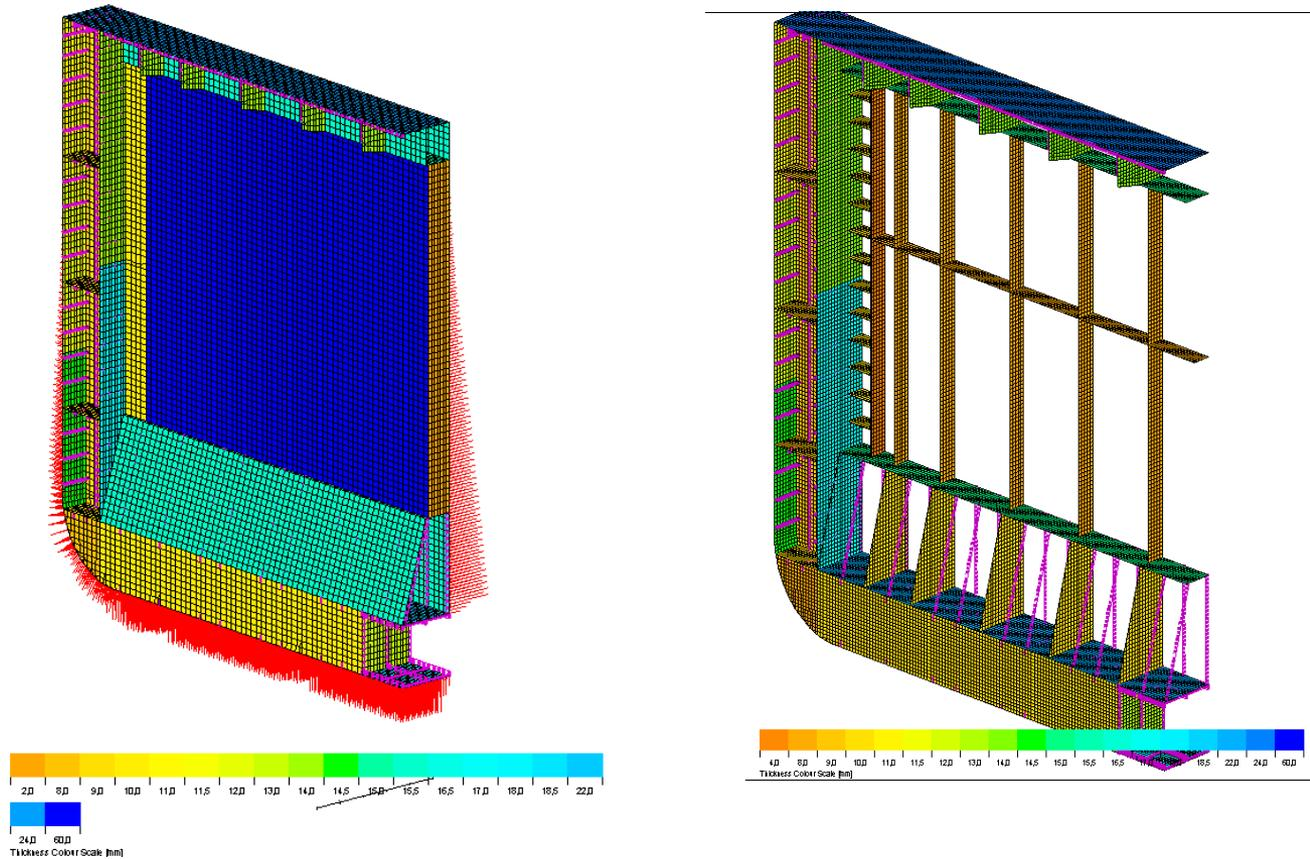
Transversal bulkhead structure FE model
