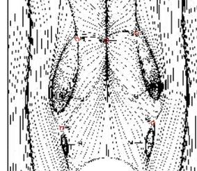
Flow topology around the cylinder in the rear side of cylinder
