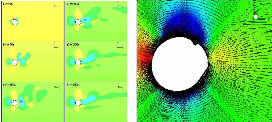
*Velocity contours at the different time      The velocity vectors existing near the cylinder*
