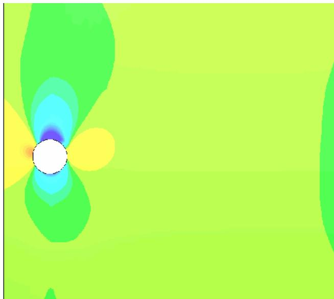
*The pressure contour around the cylinder*
