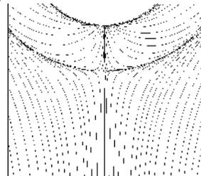
Flow topology around the cylinder in front of cylinder
