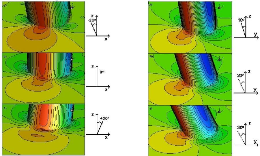
Pressure fields around a cylinder inclined longitudinally
