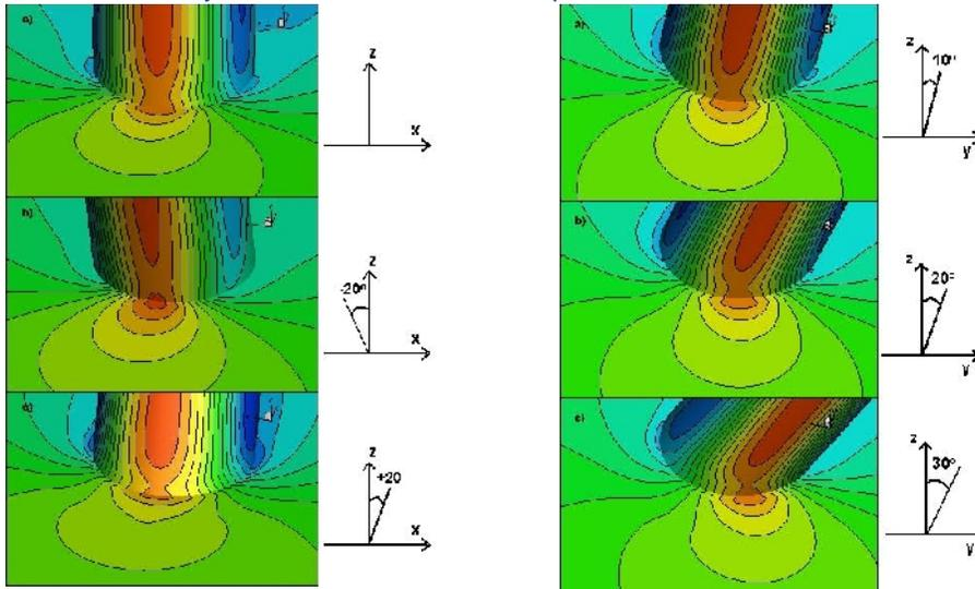
Pressure fields around a cylinder inclined longitudinally
