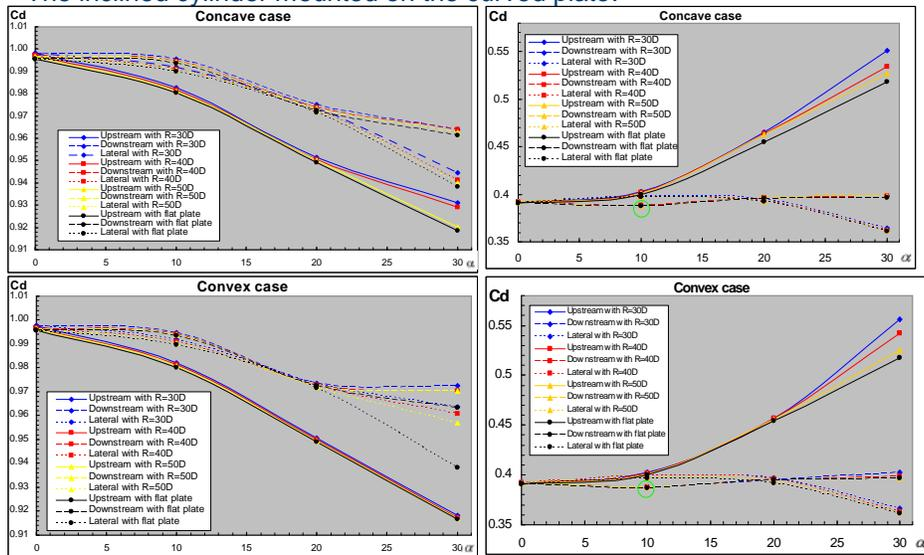
Curvature influence on the drag coefficient of the cylinder
