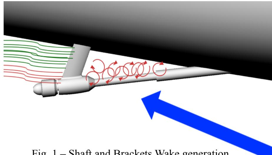
Fig. 1 – Shaft and Brackets Wake generation
