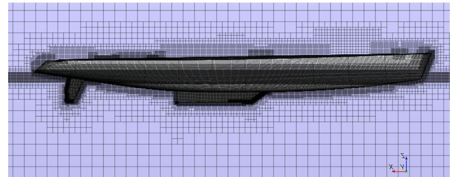
Fig.6 – Hull mesh
