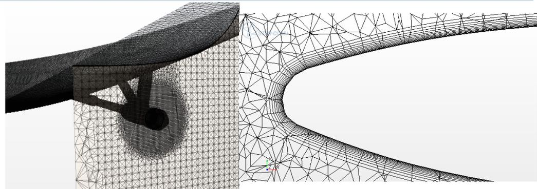
Fig. 18 – Mesh refinement and prism layer
