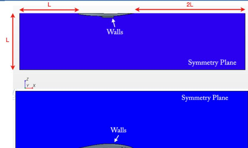
Fig. 15 – Domain of simulation (propeller performances study)
