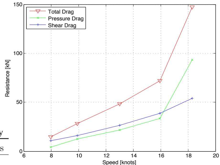
Fig.8 – Resistance [kN] as function of the Speed [knots]
