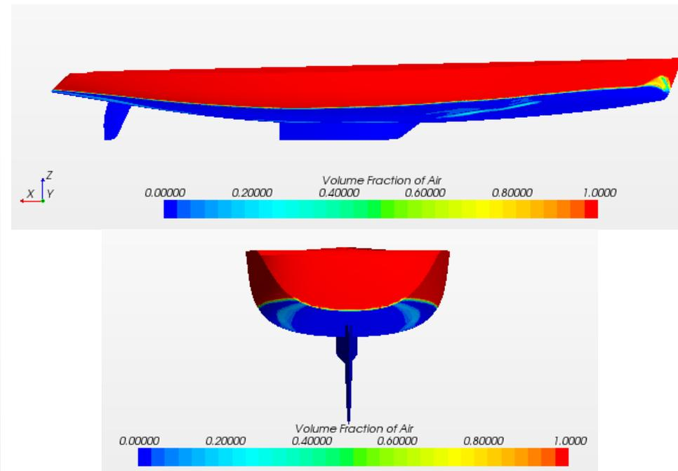
Fig. 12 – Wave pattern along the hull (18.3 knots)
