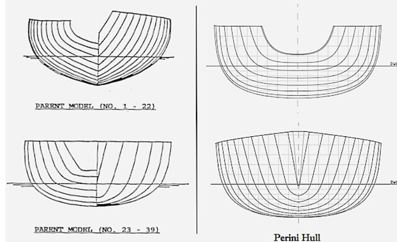
Fig. 9 – Guerritsma parent hull an Perini Navi hull
