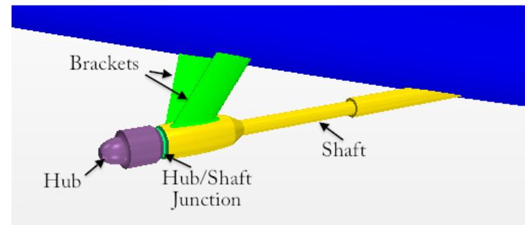
Fig. 16 – Shaft line parts
