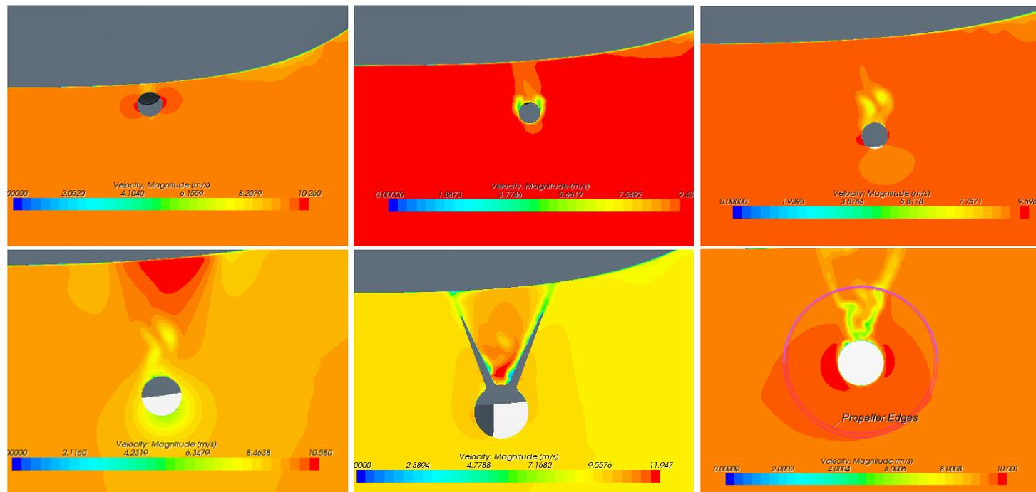
Fig. 19 – Shaft line wake steps
