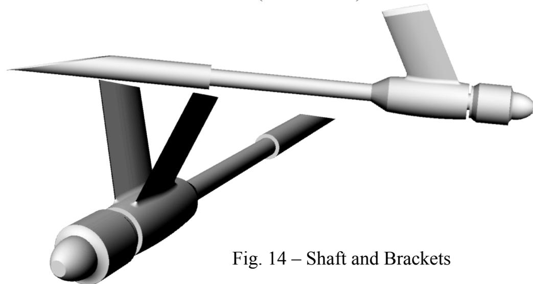
Fig. 14 – Shaft and Brackets
