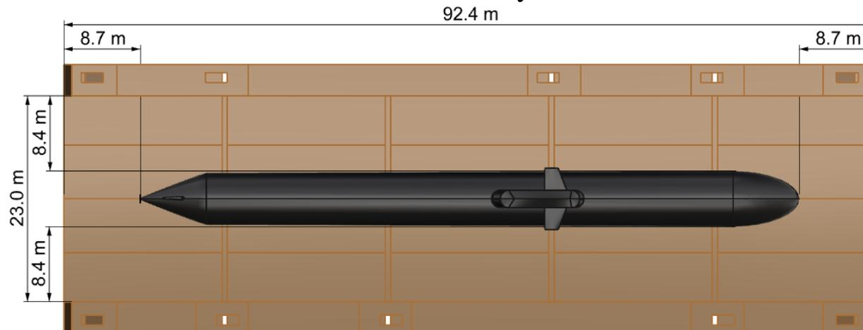
Dimensional Clearances for Scorpene Class Submarine (Top View)
