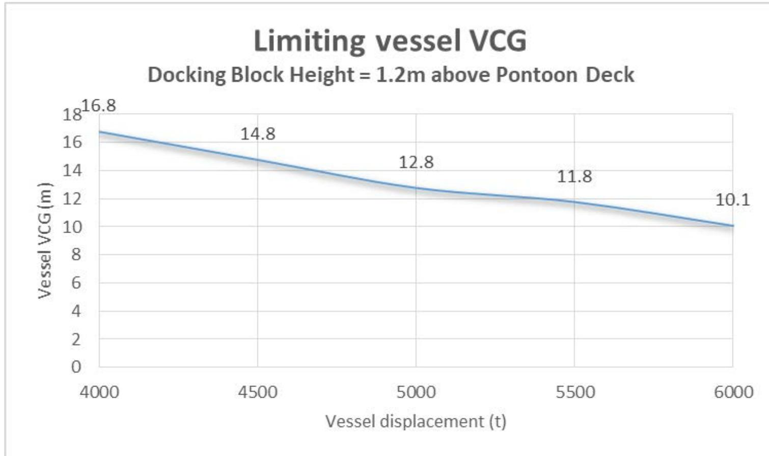
Limiting Vessel VCG-Displacement Curve
